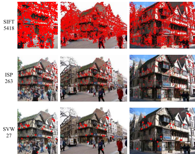
Fig. 2. The first row displays the SIFT points in 3 relevant images. The second row sets out the ISPs that occur in 3 images. For ISP_l , if d_l^i \neq \emptyset, \forall 1 \leq i \leq 3 , it occurs in 3 images. The third row shows the ISPs with CS=3 , i.e. SVWs that are accordant in 3 images. The average amount of SIFT in three images is 5418, ISP is 263, and SVW is 27.
